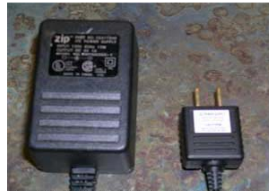
Note the dramatic size difference between the inefficient power supply on the left and the switch-mode power supply on the right
