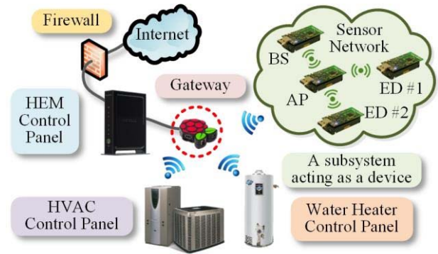
Figure 1. The hardware architecture of the HEM platform. As you may see, the “Gateway” may be eliminated, if the appliance or subsystem is capable of communicating with the platform directly.
